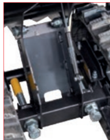
Ribaltamento manuale con pistone a gas Manual tipping with gas piston
